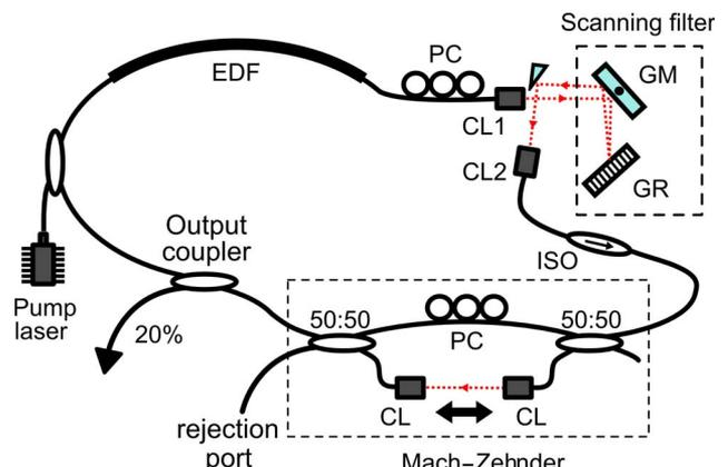
Fig. 1. (Color online) Schematic of a harmonic SFM fiber laser.
