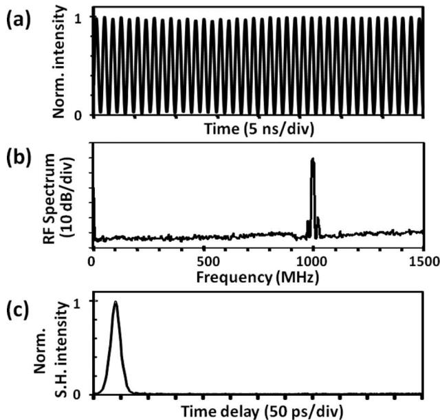
Fig. 4. (a) Pulse train from SFM laser operating at the fortieth harmonic. (b) Corresponding rf spectrum shows 1 GHz pulse repetition rate. (c) Autocorrelation shows a single peak, without the extended pedestal, indicating well-separated pulses.
