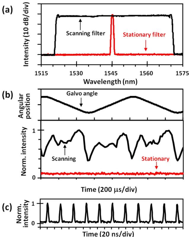
Fig. 2. (Color online) (a) Peak-hold spectrum of laser with scanning and stationary filters. (b) Peak intensity of laser emission versus position of galvanometer mirror. (c) Laser emission as measured with a 125 MHz bandwidth photodiode.
