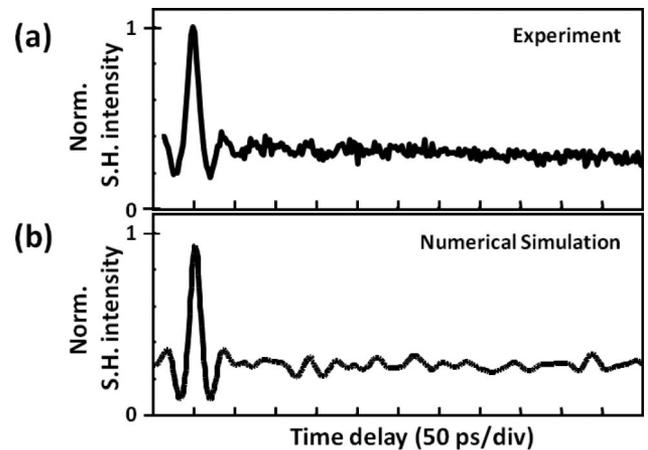
Fig. 3. Comparison of intensity autocorrelation for (a) experiment and (b) simulation. Simulation shows that the extended pedestal is consistent with multiple (e.g., 36) pulses with approximately the same amplitude and pulse width but distributed at random intervals.
