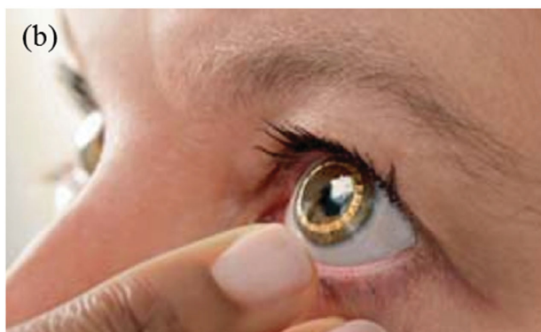
Figure 13. The SENSIMED Triggerfish holds Class IIa CE approval. a) The contact lens sensor transmits IOP measurements wirelessly to the antenna unit, which transmits the data to the data recording unit device. Data from the recording device is sent to a practitioner's computer for analysis. 1) The sensor; 2) wireless telemetry system; 3) cable that transmits data from the wireless telemetry system to the recorder unit; and 4) the data recording unit. b) The contact lens sensor worn in a human eye. Reproduced with permission. [156,157] Copyright 2013, Sensimed AG.
