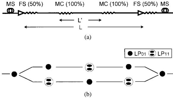
Fig. 3. (a) Schematic of the nonreciprocal comb filter with a variable comb spacing. FS: Frequency shifter. MS: LP<sub>11</sub> mode stripper. MC: Mode converter. (b) Illustration of the mode transition in the device.
