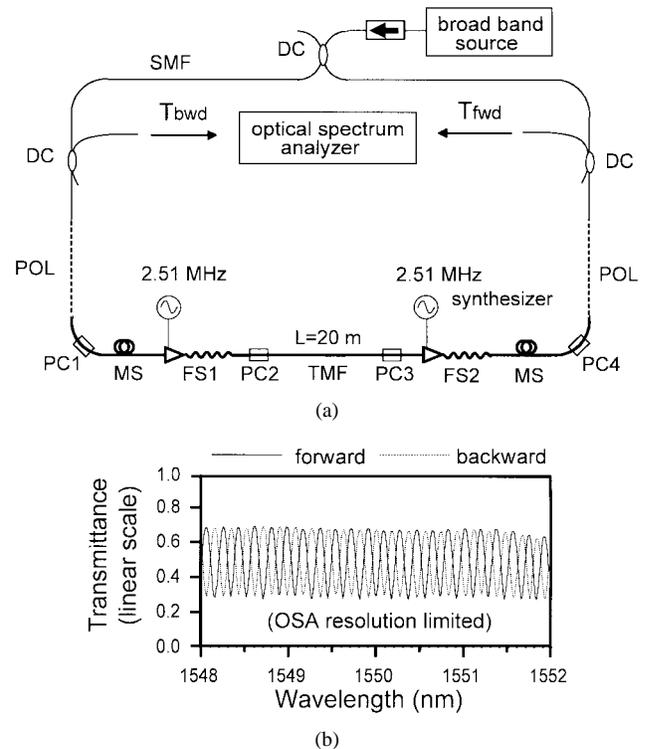
Fig. 2. (a) Experimental setup. DC: directional coupler. SMF: Single-mode fiber. TMF: Two-mode fiber. POL: Polarizing fiber. FS: Frequency shifter. MS: LP<sub>11</sub> mode stripper. PC: Polarization controller. (b) Measured transmission spectra of the comb filter.
