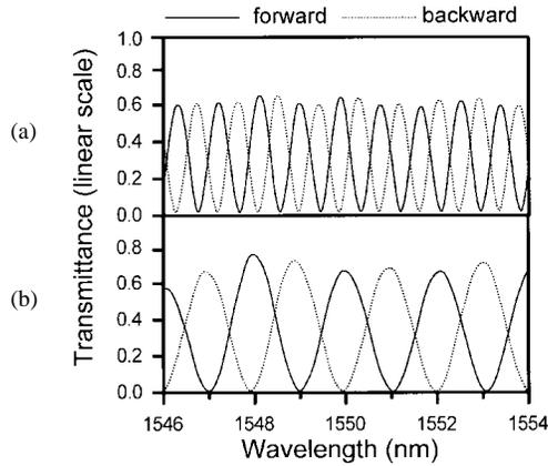
Fig. 4. Forward and backward transmission spectra of the comb filter with comb spacing adjusted to (a) 1 nm and (b) 2 nm.
