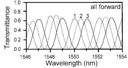
Fig. 5. Tuning of the forward transmission spectra by controlling  $\delta_a$ . Spectra 1, 2, and 3 correspond to  $\delta_a = 0, \pi/2, \text{ and } \pi$ , respectively.
