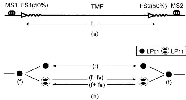
Fig. 1. (a) Schematic of the nonreciprocal device. (b) Illustration of the mode and frequency transitions in the device. TMF: Two-mode fiber. FS: Frequency shifter. MS: LP<sub>11</sub> mode stripper.
