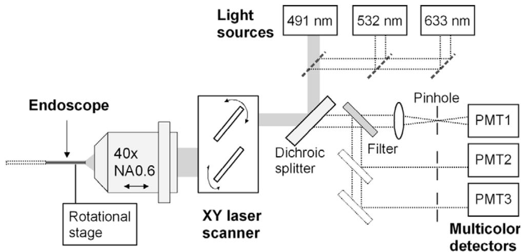
**Supplementary Figure 1:** Schematic of the imaging system. The imaging head is reconfigurable to mount the objective lens and endoscope vertically.
