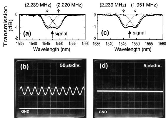
Fig. 4. Performance comparison of the conventional method using only two modes [(a) filter profile and (b) output signal] with our novel multifrequency operation using multiple modes [(c) filter profile and (d) output signal]. GND, electrical ground.
