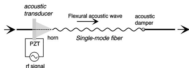
Fig. 1. Schematic of a novel all-fiber acousto-optic tunable filter. PZT, piezoelectric transducer.
