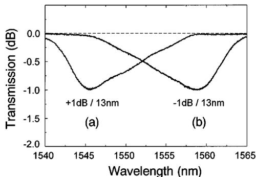
Fig. 5. Variable spectral profile of the AOTF: two examples are demonstrated with different spectral tilt coefficients.
