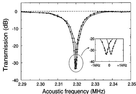
Fig. 3. Measured transmission for two eigenpolarization states of input light at  $\lambda = 1530$  nm as a function of acoustic frequency.
