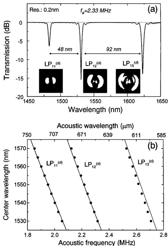
Fig. 2. (a) Transmission spectrum for a unpolarized broadband source, showing coupling to three different cladding modes [LP<sub>11</sub><sup>(cl)</sup>, LP<sub>12</sub><sup>(cl)</sup>, and LP<sub>13</sub><sup>(cl)</sup>] at an acoustic frequency of 2.33 MHz. Insets, far-field radiation patterns of the cladding modes. (b) Measured (•) and calculated (—) center wavelengths of notches as a function of acoustic frequency for couplings to three different cladding modes. Res., resolution.
