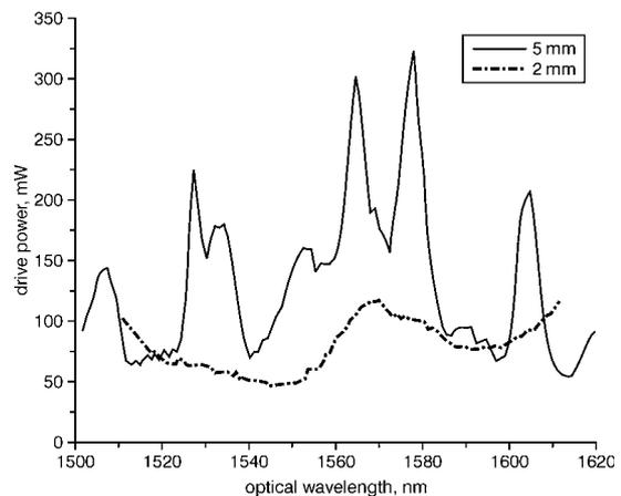
**Fig. 2** Electrical power consumption of two devices with different transducer diameters
