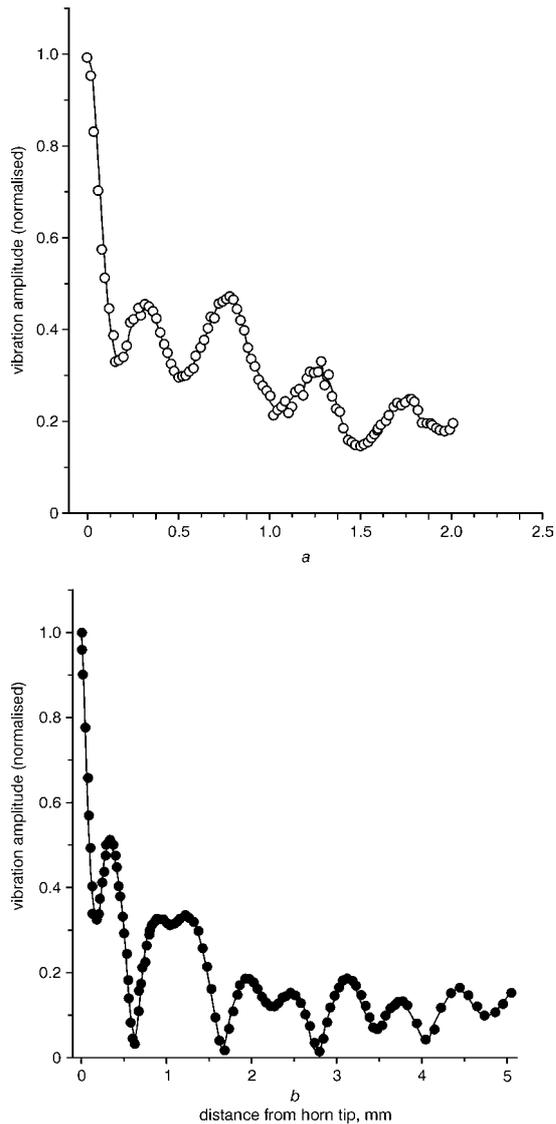
**Fig. 3** Acoustic amplitude along surface of horn for different transducer diameters
