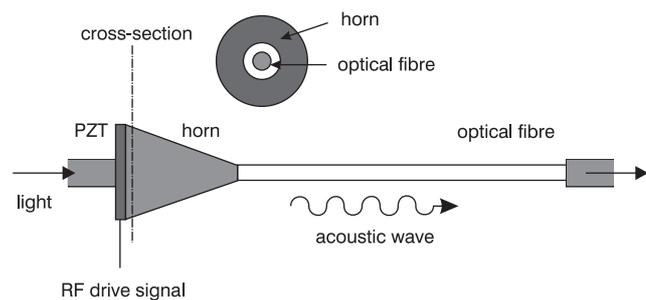
**Fig. 1** Schematic of fibre-based acousto-optic filter with coaxial acoustic transducer
