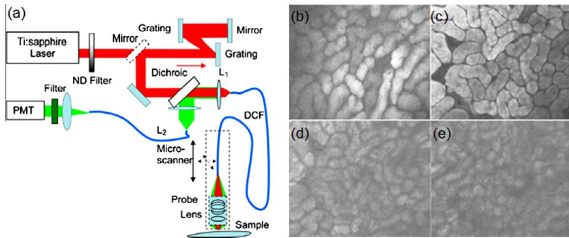
**Fig. 7.** Microendoscope based on double-clad fiber. (a) Schematic of two photon fluorescence endoscopic system. (b)–(e) Two photon fluorescence images of a rat kidney surface. 0, 20, 40, 60  $\mu\text{m}$  deep from the surface. (From Bao, H., et al., *Fast handheld two-photon fluorescence microendoscope with a 475  $\mu\text{m}$   $\times$  475  $\mu\text{m}$  field of view for in vivo imaging*. Optics letters, 2008. 33(12): p. 1333–1335; with permission) [46].
