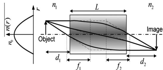
**Fig. 10.** Refractive index profile and image formation of a GRIN lens. (From Fu, L. and M. Gu, *Fibre-optic nonlinear optical microscopy and endoscopy*. *Journal of Microscopy*, 2007. 226(3): p. 195–206; with permission) [14].
