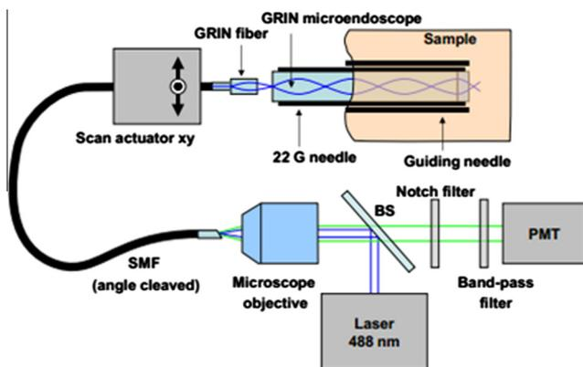
**Fig. 4.** The schematic of confocal microendoscope based on single-mode fiber. BS: dichroic beamsplitter, PMT photomultiplier tube. (From Pillai, R.S., D. Lorenser, and D.D. Sampson, *Deep-tissue access with confocal fluorescence microendoscopy through hypodermic needles*. Optics Express, 2011, 19(8): p. 7213–7221; with permission) [32].
