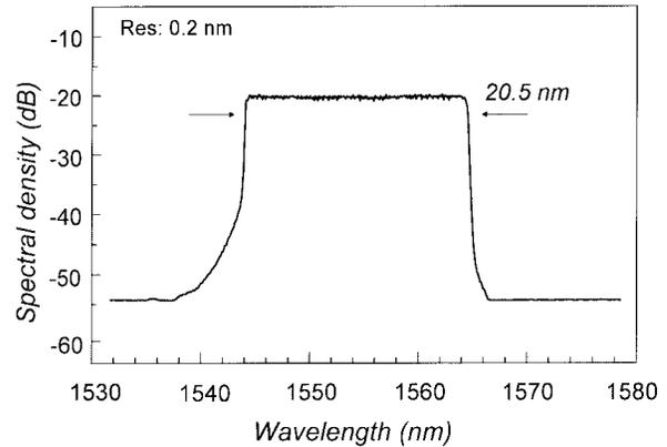
Fig. 9. Peak-hold output spectrum swept over 20 nm by an acoustic frequency sweep over 1 MHz around 68 MHz with a fixed acoustic power.
