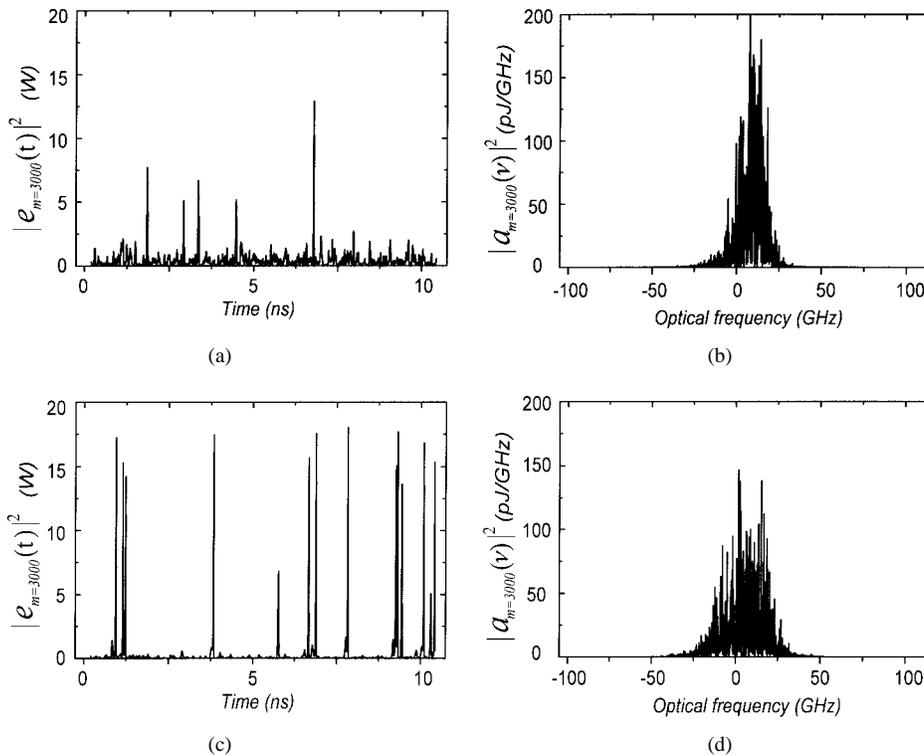
Fig. 3. Simulation results for the spectral and temporal power densities at a laser output power of 10 mW. Temporal results: (a) and (c), spectral results: (b) and (d). The ASE spectral power densities used were  $1.723 \cdot 10^{-23}$  J/Hz for (a) and (b), and  $1.723 \cdot 10^{-25}$  J/Hz for (c) and (d), respectively.
