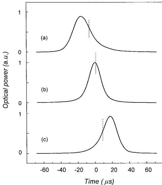
Fig. 4. The laser output on reflection from a narrow-band fiber grating at a sweep frequency of (a) 250 Hz, (b) 270 Hz (close to the resonant sweep), and (c) 290 Hz. Its temporal width is related to the laser linewidth. The dotted lines indicate the filter peak wavelengths. The anticipated spectral asymmetry is evident in (a) and (c) [Fig. 1].
