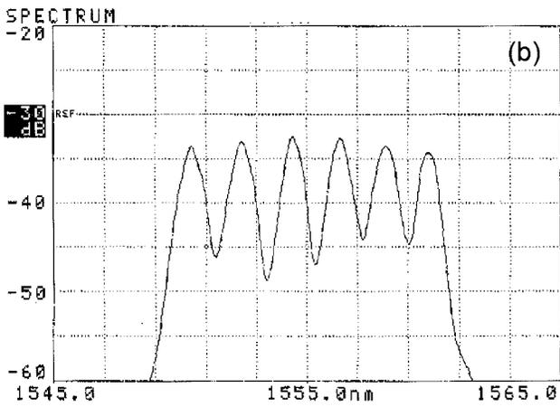
Fig. 11. (a) The laser output in the time domain at a 9.3-kHz sweep rate (lower trace). The upper trace is a modulation signal applied for the acoustic frequency sweep. (b) Max-hold spectrum.
