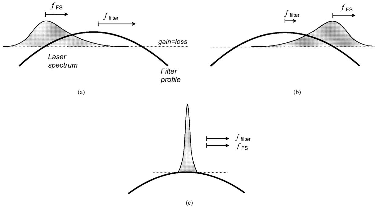
Fig. 1. Schematic of the laser spectrum in a wavelength swept laser when (a)  $f_{\text{filter}} > f_{\text{FS}}$ , (b)  $f_{\text{filter}} < f_{\text{FS}}$ , and (c)  $f_{\text{filter}} = f_{\text{FS}}$ .
