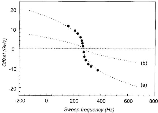
Fig. 6. Offset frequencies at (a) 3-mW and (b) 100-mW output power levels as a function of sweep frequency for the 20-nm total wavelength sweep (data points: experimental values, dashed lines: numerical simulations).
