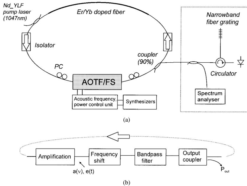
Fig. 2. (a) Experimental fiber laser with a spectral analysis setup. (b) Schematic diagram of the laser used in the computer simulation.
