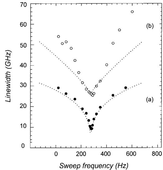
Fig. 5. Linewidths at (a) 3-mW and (b) 100-mW output power levels as a function of sweep frequency for the 20 nm total wavelength sweep (data points: experimental values, dashed lines: numerical simulations).
