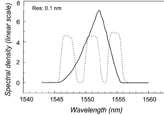
Fig. 12. Triangular (solid line) and square (dotted line) modulated output spectra obtained by synchronous modulations of the filter transmission and peak wavelength.
