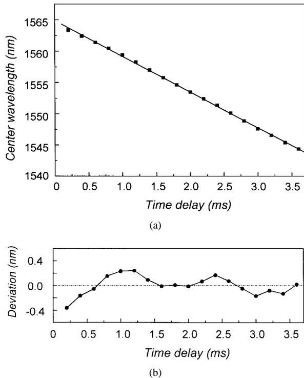
Fig. 8. (a) Time-varying output center wavelength for the 20-nm sweep at 270 Hz. The solid line is a linearly fitted curve. (b) Deviation of the experimental values from the linear fit curve.
