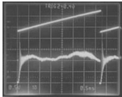
Fig. 10. Laser output in the time-domain (lower trace) when the filter peak is modulated over 20 nm by a saw tooth wave input to the AOTF drive system (upper trace). Significant relaxation oscillation is observed at the beginning of each sweep but dies down within a short fraction of the full sweep.
