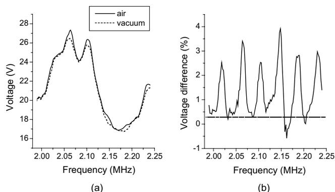
Fig. 4. (a) Voltages for 5-dB notch depth in the air and vacuum. (b) Voltage increase by the air. Dotted line: background voltage increase.
