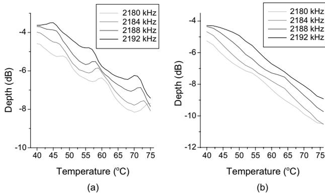
Fig. 2. Notch depths measured as a function of temperature and acoustic frequency (a) with and (b) without the metal tube.
