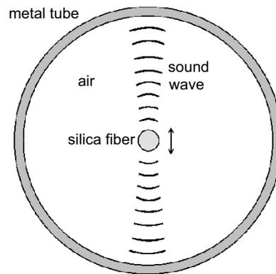
Fig. 3. Resonance of sound wave inside the metal tube.
