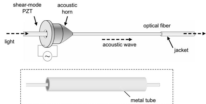
Fig. 1. Schematic of the fiber-based acoustooptic filter. Inset: packaged device with metal tube.
