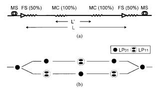
Fig. 3. (a) Schematic of the nonreciprocal comb filter with a variable comb spacing. FS: Frequency shifter. MS: LP11 mode stripper. MC: Mode converter. (b) Illustration of the mode transition in the device.
