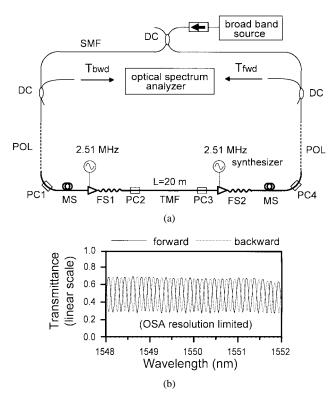
Fig. 2. (a) Experimental setup. DC: directional coupler. SMF: Single-mode fiber. TMF: Two-mode fiber. POL: Polarizing fiber. FS: Frequency shifter. MS:  $LP_{11}$  mode stripper. PC: Polarization controller. (b) Measured transmission spectra of the comb filter.
