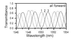
Fig. 5. Tuning of the forward transmission spectra by controlling  $\delta_a$ . Spectra 1, 2, and 3 correspond to  $\delta_a = 0, \pi/2$ , and  $\pi$ , respectively.
