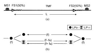
Fig. 1. (a) Schematic of the nonreciprocal device. (b) Illustration of the mode and frequency transitions in the device. TMF: Two-mode fiber. FS: Frequency shifter. MS:  $LP_{11}$  mode stripper.
